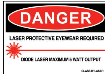
Figure 7.1 Label to be posted at entrance to treatment area
