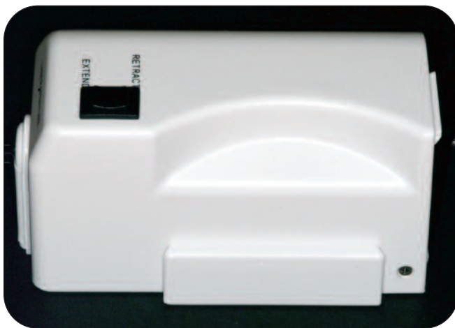
Figure 3.11 Disposable Fiber Cassette without the End Cap
