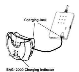
NOTE: Charging jack of BAG-2000 is able to using ear-set jack with jumper setting from inside BAG-2000.
