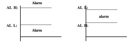
Pressing the menu button(3), then "AL H: 0C" is displayed on LCD monitor. ("C"(Celsius) or "F"(Fahrenheit) is displayed on LCD monitor. It was selected before) And then you change value by using up(5) or down(6) button.
