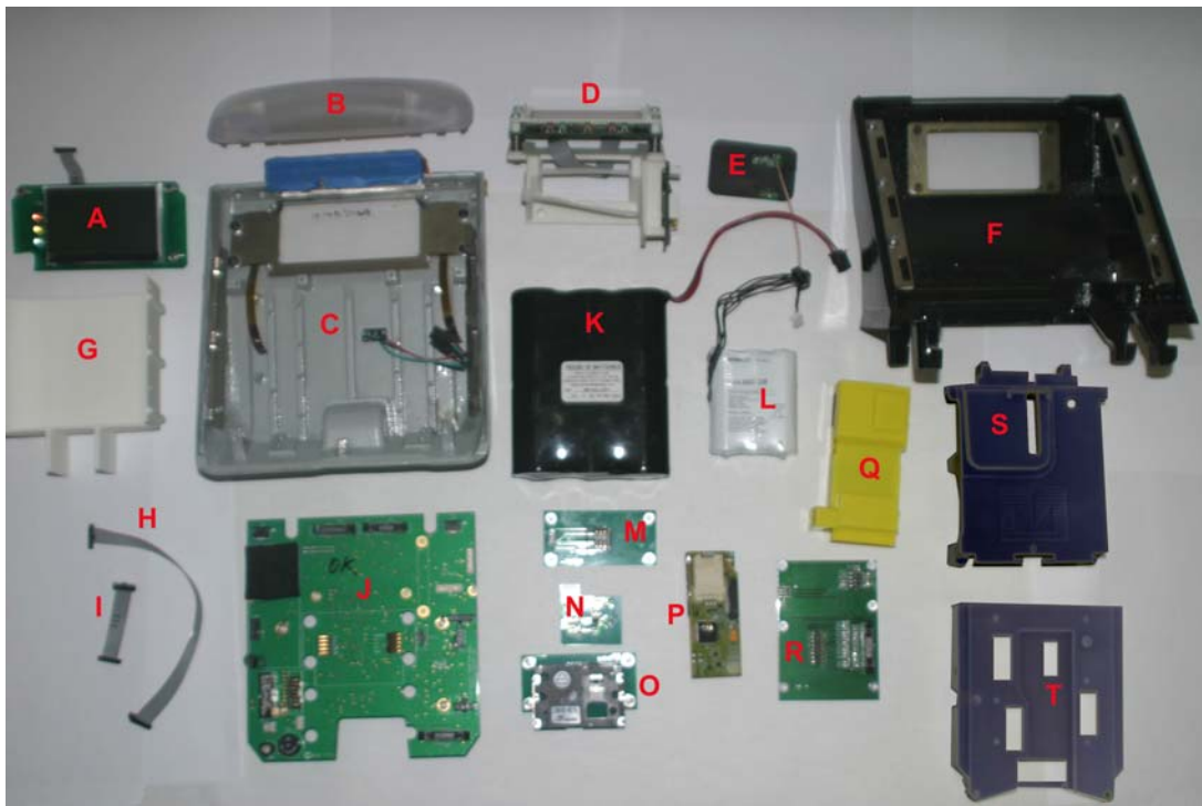
• Figure 7 – Exploded Parts View of the Mackay Guardian™ Solo
