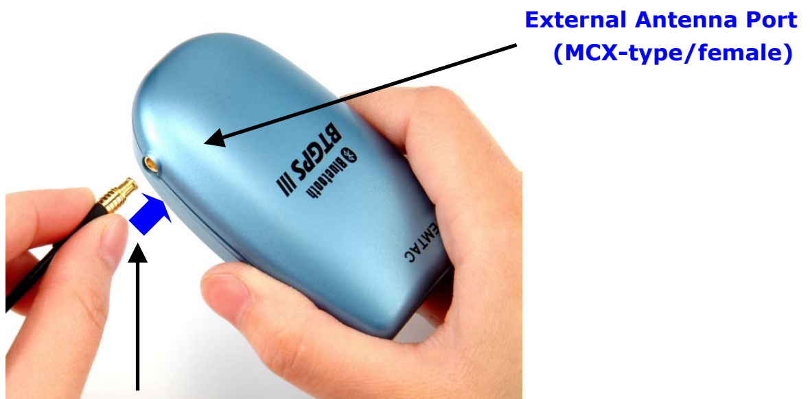
Connector of the optional External Active Antenna (MCX-type/male)
