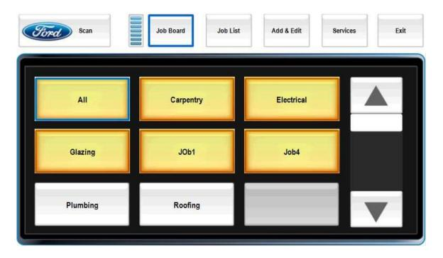
ToolLink opens up in the Job Board screen, which provides an overview of tool inventory. Each group of tools has its own button. Red buttons indicate that tools are missing from a group. Silver buttons indicate that all tools are present.
