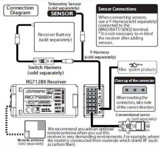
Note: After adding a remote antenna you must re-bind to ensure correct functionality.
