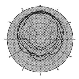
Composite octave polar responses of the 2152H in both horizontal and vertical planes over the range of 500 Hz to 16 kHz (1 meter measurement distance in an anechoic chamber).
