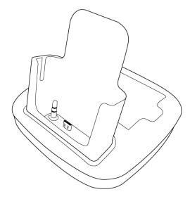
Place the cradle on a desk or table top so that the ports are facing to the back. There is a tall rectangular protusion facing toward you into which you can insert the Blaze EZ. Inside this compartment are 2 connectors. On the left is an audio connector and on the right is a micro USB connector. To use the Blaze EZ in the cradle, slide it into the compartment with the keyboard facing toward you. Gently press down until you feel the connectors engage.
