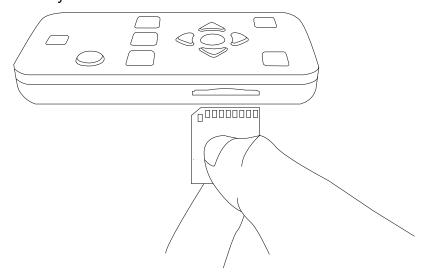
To remove the SD card, gently press the SD card into the card slot until it clicks, then release it. The SD card will pop out of the slot enough for you to grip it and pull it out completely. If the Blaze EZ is turned on, you will hear a sound to confirm that it has detected the removal of the SD card followed by the announcement, "SD card removed".
