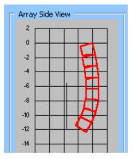
Figure #10. : Side View of 8-Box VT4889 Array, configured as a progessive line array
