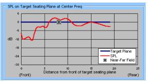
Figure 8. : Predicted SPL on 2k Hz center frequency. Front seating rows at left.
