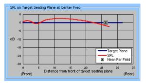
Figure #12. : Predicted SPL on balcony seating plane, 2 kHz
