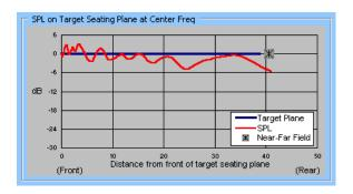
Figure #11. : Predicted SPL on main floor seating plane at 2K Hz center frequency.
