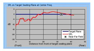
Figure #15. : Predicted SPL on main floor seating plane at 2k Hz center frequency, in venue with very high suspended arrays.
