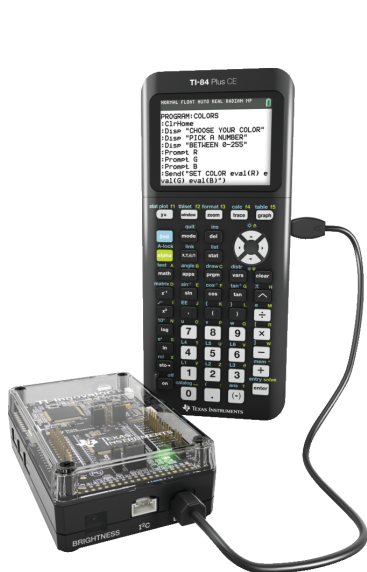
Hub connected to TI CE Graphing Calculator
