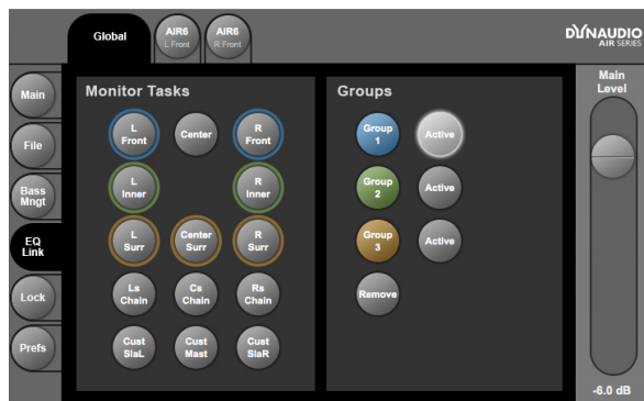
Fig. 43: AIR Control software – Global – EQ Link page. Group 1 (containing the left and right front speakers) is active.
