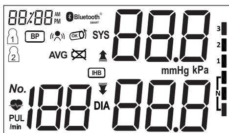
Note: Unit will not function if residual air from previous testing is present in cuff. The LCD will flash "↓" until pressure is stabilized.
