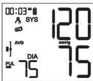
Press the "MEM" button again, you may check past test results. Upon activating test results, you can press the "MEM" button to scroll through all test results stored in memory. The LCD will display the last memory as NO: 01 reading. ("MEM" button means turn forward)
