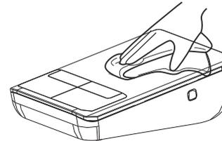
4. **Cuff Cleaning:** Do not soak cuff in water! Apply a small amount of rubbing alcohol to a soft cloth to clean cuff's surface. Use a damp cloth (water-based) to wipe clean. Allow cuff to dry naturally at room temperature. The cuff must be cleaned and disinfected before use between different users.
