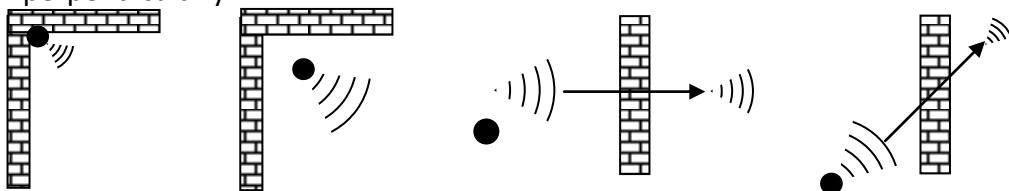
Waves cannot pass through full metallic walls. On the other hand, a perforated wall allows the waves passing with attenuation
