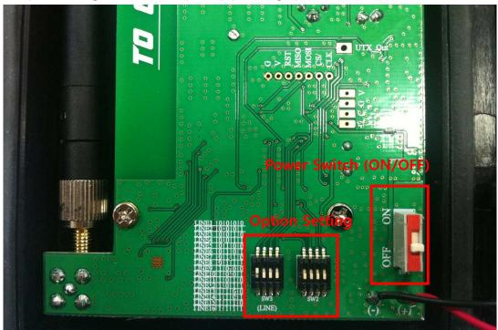
As shown in the photo above, there are two option switches inside the CURBTX unit. The switch on the left is to select a parking space (line) among the 16 spots assigned in the PC program, and the one on the right is to add additional options.
