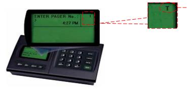
Transmit Indicator – page being sent using keypad or thru RS232 port. This also indicates the Out of Range signal is being sent.
