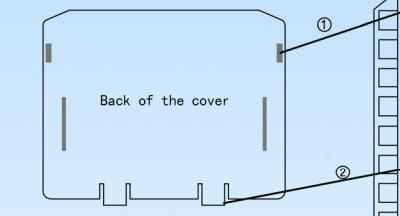
2. Insert the points (1) into the holes as arrow aheaded, press down slightly. Press points(2) into the holes as arrow aheaded.
