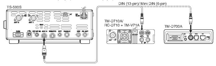
After connecting the 2 transceivers with the cable, access Menu Nos. 73 (PKS polarity) and 74 (Busy lockout) on the TS-590S transceiver and select "on". You will further need to adjust the audio input/ output level of the TS-590S transceiver using Menu Nos. 66 and 67.
