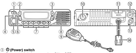
Press to switch the transceiver ON or OFF.
