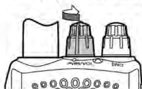
Turn the **PWR/VOL control** counterclockwise to switch the transceiver OFF.
