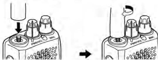
**Note:** The antenna is neither a handle, a key ring retainer, nor a speaker/ microphone attachment point. Using the antenna in these ways may damage the antenna and degrade your transceiver's performance.
