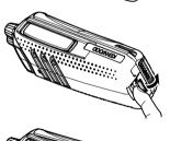
2 To remove the battery pack, lift the safety catch on the base of the transceiver, then press the release latch underneath the safety catch.
