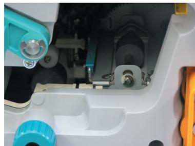
2. With the guard component (green color) on your right, turn the inverter vertical with your hand. Turning the inverter will move the card away from its center. As such, turn the jog dial to return card to the center of the inverter while you are turning the inverter.
