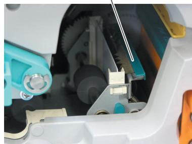
3. Turn the jog dial to move card to the top and remove with hand.
