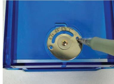
During printing, when the card is not discharged from the card cassette, adjust the gate adjustment position clockwise, one scale at a time. If 2 cards are discharged, adjust the gate adjustment position anti-clockwise.
