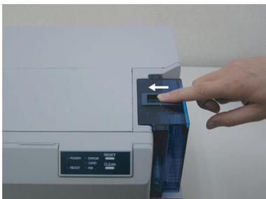
Lift the card cassette up by about 1cm and slide to the right to remove the cassette.
