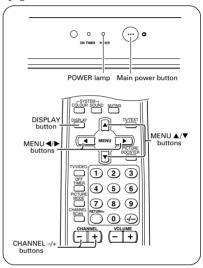
To stop the AUTO PROGRAMMING function, press the CHANNEL -/+ or the MENU
