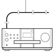
When good radio reception cannot be obtained with the supplied antenna or when using a communal antenna
