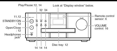
\* Connect a pair of headphones (commercially available) with a stereo mini plug. If the headphones are connected, the speakers and subwoofer will not produce any sound.
