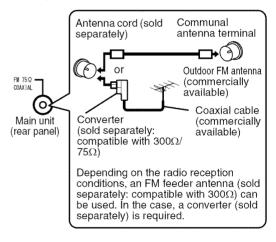
For details of connecting a separately sold antenna, refer to the user guide for the antenna or converter.
