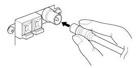
If reception is poor, connect the outdoor antenna.
