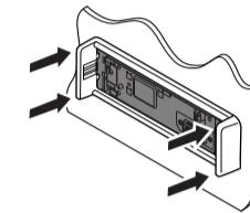
Fit the receiver into the mounting sleeve by using four corners of the trim plate.
