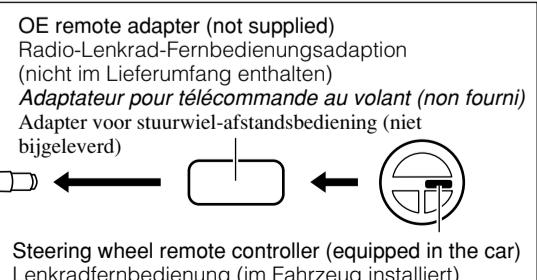
Steering wheel remote controller (equipped in the car)
