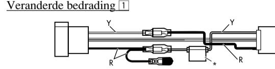
Use modified wiring 1 if the receiver does not turn on.
