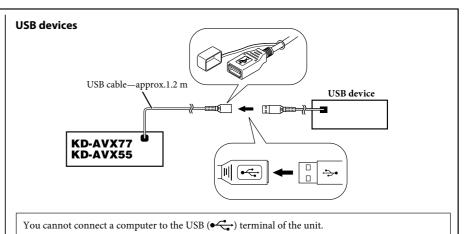
Connecting the iPod or iPhone device to the USB terminal
