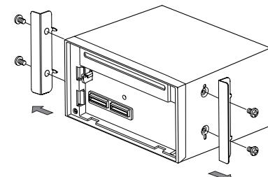
Remove the metal protection plates from the unit before installation.
