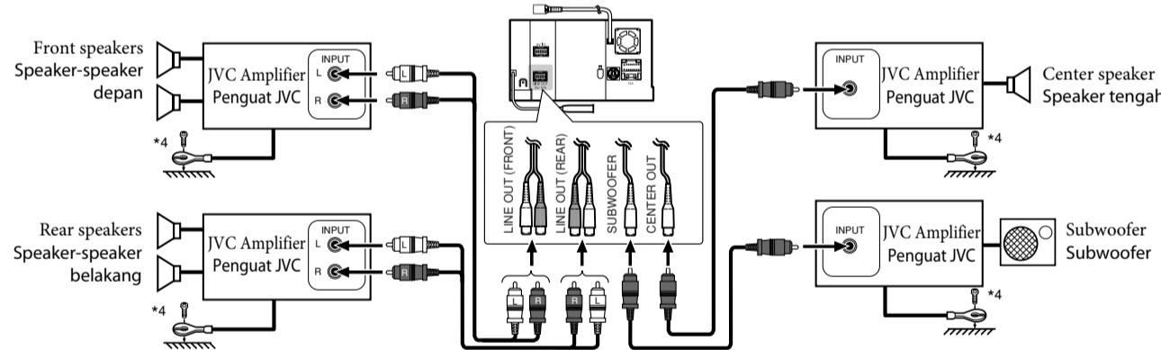
\*4 Firmly attach the ground wire to the metallic body or to the chassis of the car—to the place uncoated with paint (if coated with paint, remove the paint before attaching the wire). Failure to do so may cause damage to the unit.
