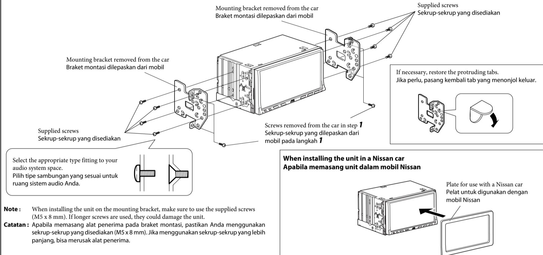
**Note :** When installing the unit on the mounting bracket, make sure to use the supplied screws (M5 x 8 mm). If longer screws are used, they could damage the unit.
