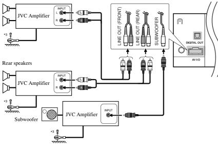
\*3 Firmly attach the ground lead to the metallic body or to the chassis of the car—to the place uncoated with paint (if coated with paint, remove the paint before attaching the lead). Failure to do so may cause damage to the unit.
