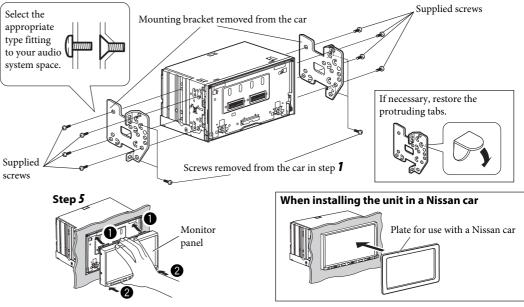
When installing the unit on the mounting bracket, make sure to use the supplied screws (M5 x 8 mm). If longer screws are used, they could damage the unit.
