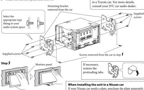
· When you use screws other than those supplied, use 8 mm-long screws. If longer screws are used, they could damage the unit
