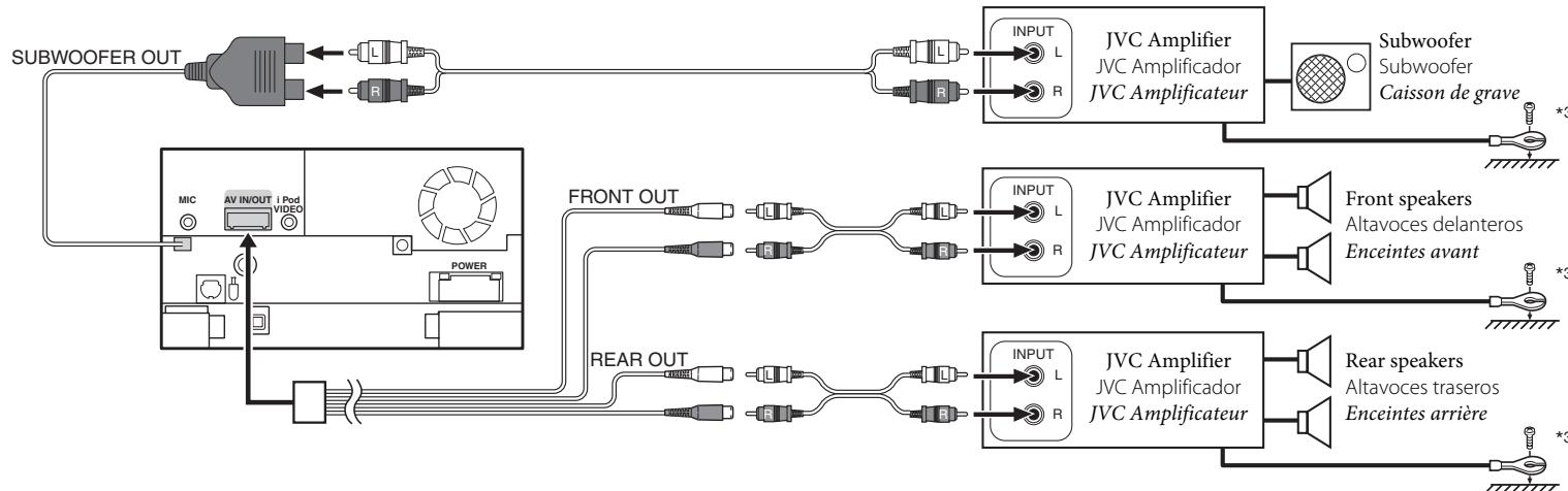
\*<sup>3</sup> Firmly attach the ground lead to the metallic body or to the chassis of the car—to the place uncoated with paint (if coated with paint, remove the paint before attaching the lead). Failure to do so may cause damage to the unit.
