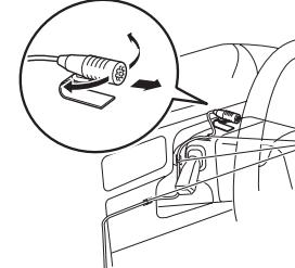
Secure the microphone cord using cord cramps (not supplied) if necessary.
