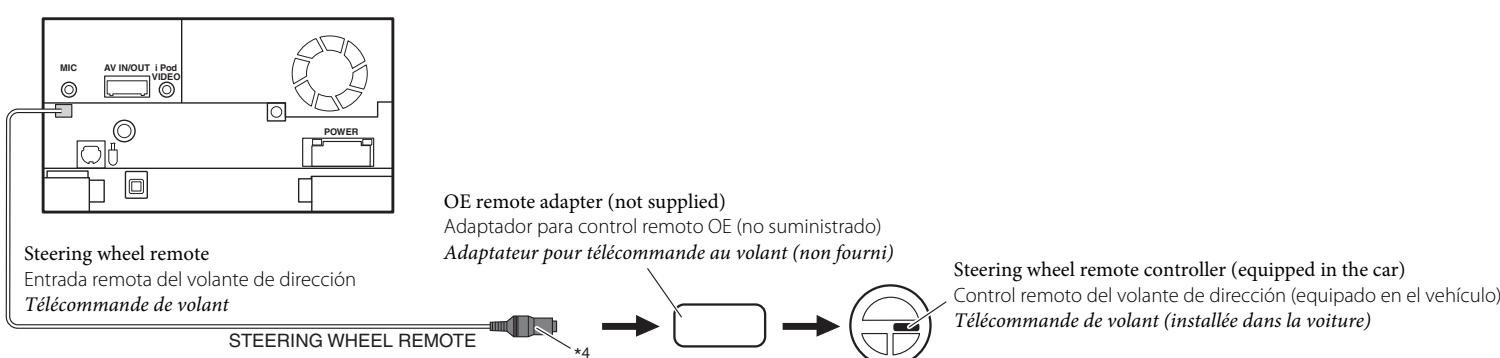
\*<sup>4</sup> If your car is equipped with the steering wheel remote controller, you can operate this unit using the controller. For connection, an exclusive remote adapter (not supplied) which matches your car is required. For details, consult the same car audio dealer as where the unit is purchased.
