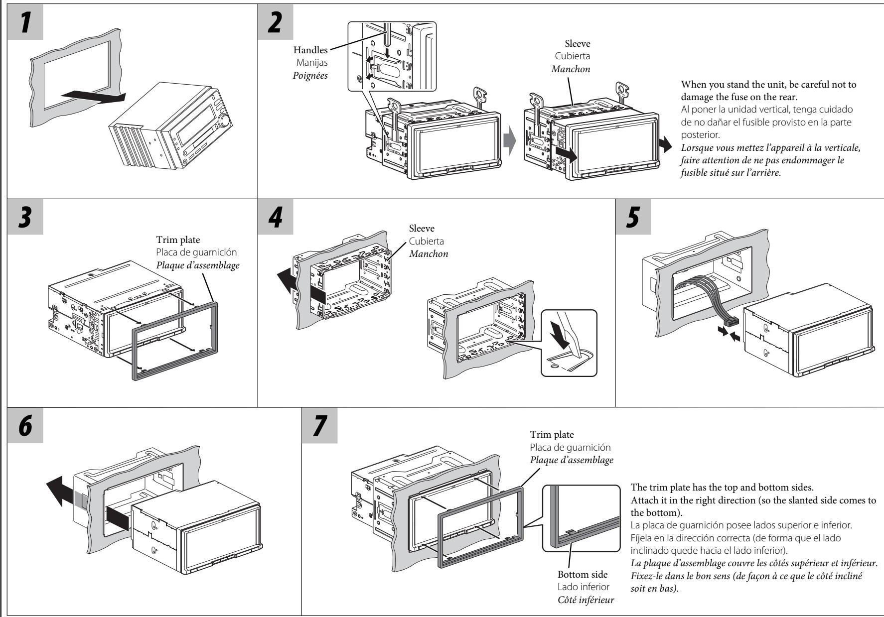
Install the unit at an angle of less than 30° vertically and of less than 5° horizontally.
