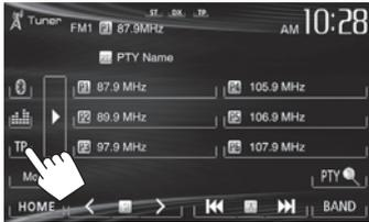
The unit is in standby to switch to Traffic Announcement (TA) if available. (The TP indicator lights up.)
