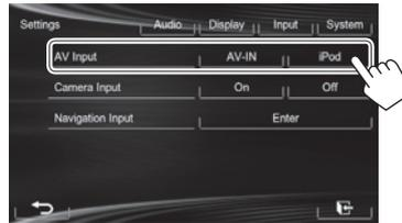
**[AV-IN]** Select this when the iPod/iPhone is connected using the USB 2.0 cable (accessory of the iPod/iPhone).
