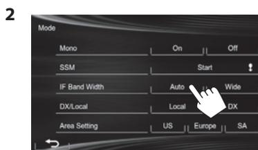
**[Auto]** Increases the tuner selectivity to reduce interference between adjacent stations. (Stereo effect may be lost.)
