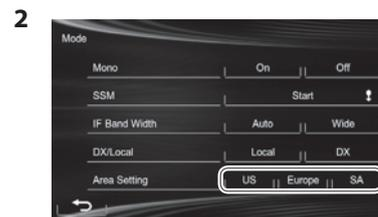
**[US]** Select this when using in North/Central/South America. FM/AM intervals are set to 200 kHz/10 kHz.
