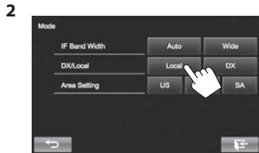
**[Local]** Select this to tune in only to stations with sufficient signal strength. The LO indicator lights up.
