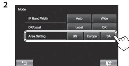
**[US]** Select this when using in North/Central/South America. FM/AM intervals are set to 200 kHz/10 kHz.
