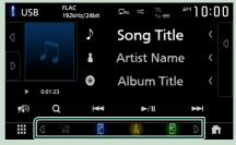
Display source selection buttons by touching / or flicking left or right on the source control screen, then select a playback source.
