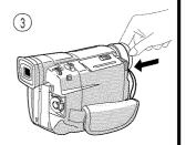
To protect the lens, attach the provided lens cap to the camcorder as shown in the illustration.
