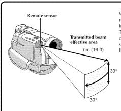
When using the remote control, be sure to point it at the remote sensor. The illustration shows the approximate transmitted beam effective area for indoor use. The transmitted beam may not be effective or may cause incorrect operation outdoors or when the remote sensor is directly exposed to sunlight or powerful lighting.
