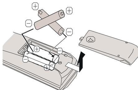
**NOTE:** Remove the batteries from remote control when it is not to be used for a long period. Otherwise it can be damaged due to any leakage of battery.
