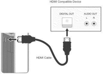
Connect the HDMI Cable from the DIGITAL OUT on the back of your DTV or HDMI device, to
