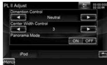
**[Dimension Control]** Sets the surround position by adjusting the front and rear volume balance.
