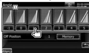
**1** Sets the Monitor angle. **[Off Position]** Stores the current monitor angle as the angle during power off.
