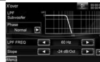
**[Phase]** Sets the phase of subwoofer output. The phase is reversed 180 degrees when set to "Reverse". (Only when "Subwoofer" is set to any item other than "None" in Speaker Setup)
