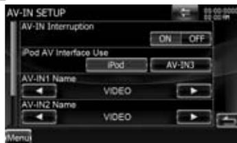
**[AV-IN Interruption]** Sets an image display of the system that is connected via the AV INPUT port. ( "OFF")
