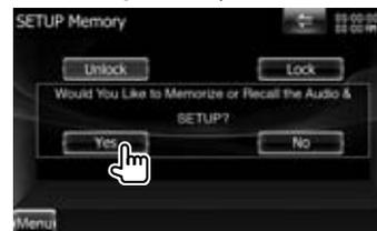
**[Lock]** Locks the AV-IN SETUP, Navigation, and Audio SETUP settings. When [Lock] is selected, you cannot change the AV-IN SETUP, Navigation,
