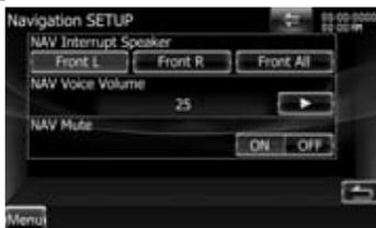
**[NAV Interrupt Speaker]** Selects speakers used for voice guidance of the navigation system.
