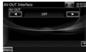
**[AV-OUT]** Selects an AV source to be output at the AV OUTPUT port. ( "VIDEO1")
