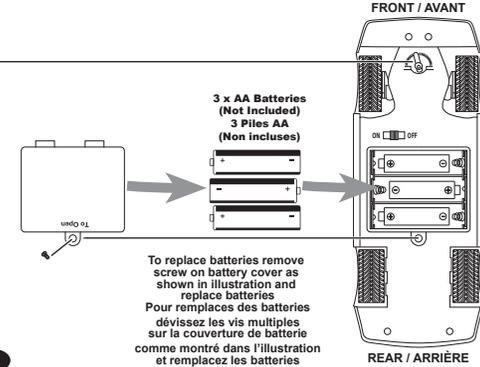
**To replace batteries remove screw on battery cover as shown in illustration and replace batteries**
