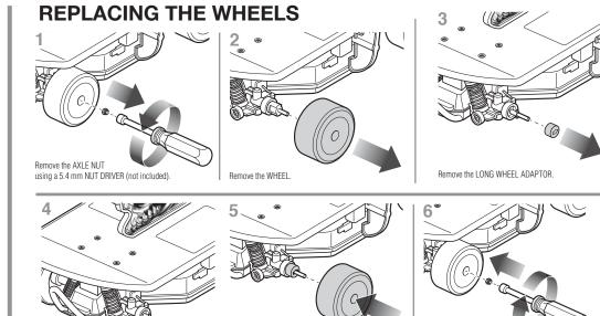
Insert a SHORT WHEEL ADAPTOR (included) onto AXLE HUB. "Wheel: Outside diameter: 1.45" (37mm); Width: 1.18" (30mm); Tires: Outside diameter: 2.39" (59mm); Width: 1.18" (30mm)
