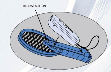
Insert the Controller into the handle, wrist strap end first. Press the top of the Controller down into the handle until you hear a "click". Be sure the wrist strap properly protrudes from the end of the accessory handle.
