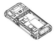
Insert the microSD card with the golden contacts facing downwards into the slot. To remove the microSD card, gently press and slide it out.
