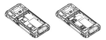
To install, place the SIM card with the chip facing downwards into the housing and slide it into its slot. Make sure that it is correctly inserted. To remove the card, press and slide it out.
