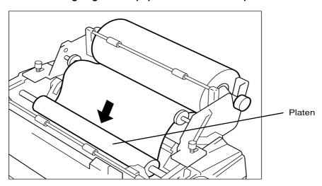
5. Turn the paper feed knob and pull out the leading edge of the paper.
