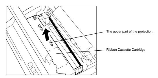
3. Turn the cassette knob of the new ribbon cassette cartridge counterclockwise to increase the tension of the ribbon.
