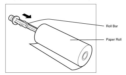
2. Attach the roll bar with the paper roll onto the paper roll stand unit holder, taking care to notice he paper roll's direction.
