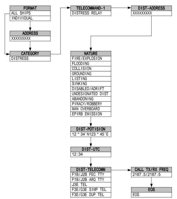
Example: Procedure of a distress relay call to all ships
