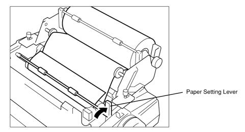
9. First, insert the axis of the left side of the paper roll cover into the left hole of the paper roll stand, then set the right side.
