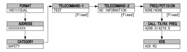
1. From the "MENU#1-EDIT&CALL" screen, press 1 1, and then press ENT. The "TEST CALL" screen is displayed.
