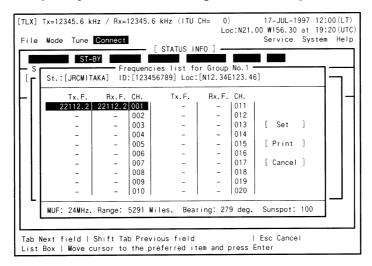
4. After the following window opened, check the channel condition and if not occupied, press Enter key.
