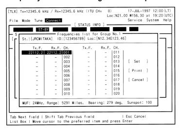
4. After the following window opened, check the channel condition and if not occupied, press Enter key.
