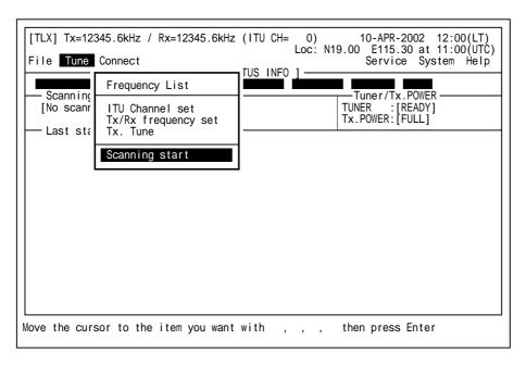
2. Select the desired station on the following window and press Enter key. Scanning is started in order by the channel number.
