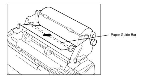
4. Insert the leading edge of the paper from behind the platen
