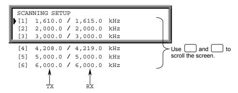
6. Enter the "Transmit frequency/Receive frequency" pair for each channel.
