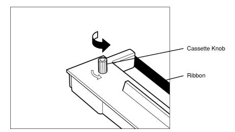
4. Manually, move the printing head to the home position (left side) and place the ribbon cassette cartridge in the printer so that the ribbon is positioned between the ribbon mask and the printing head. In this case, make sure that the ribbon feed axis is inserted through the hole under the ribbon cassette knob.
