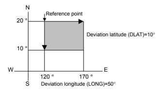
First, select the direction from N.E. (North-East), N.W. (North-West), S.E. (South-East), and S.W. (South-West). In this example, the direction is N.E.
