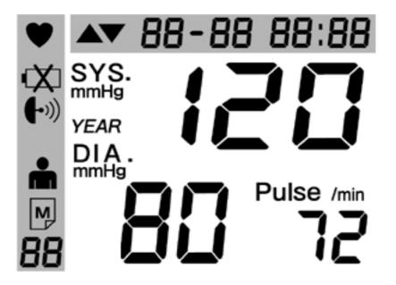
▲ Pressurization : Displays during inflation▼ Exhausting : Displays during deflation
