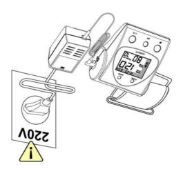
Connect the AC adapter between unit and wall outlet
