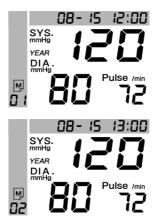
Note 1.Data saved in memory can be all deleted, exchange battery or remove an AC adapter
