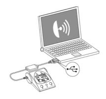
To install an USB driver in a computer, follow the guidance contained in, manual of software 'Hour 24' Turn on the power of two appliances after connecting ECHO-FT to the computer running 'Hour 24' (USB cable should be used the one supplied by JAWON MEDICAL exclusively)
