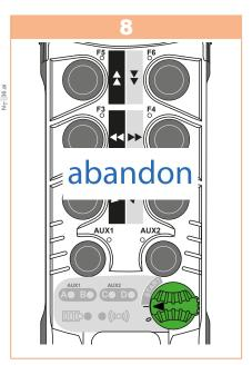
If the receiver does not receive the ID code within **20 sec** following switching the **ON/OFF** to **START**, the receiver aborts the pairing.
