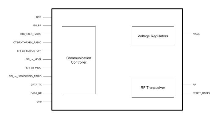
The module contains a communication controller with embedded proprietary protocol software, a narrow band high performance RF transceiver and three internal voltage regulators.
