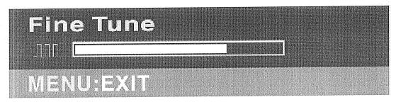
Fine Tune: To adjust the delay time.
