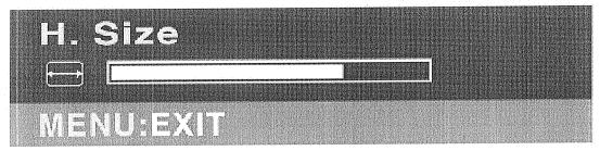
H. Size: To adjust the delay time between horizontal synchronous signal and video.
